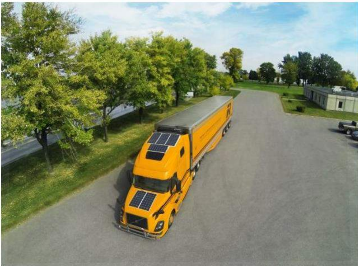
Canada's Groupe Robert is using six solar panels and four deep-cycle batteries to keep drivers comfortable and batteries charged. Photo: Groupe Robert
