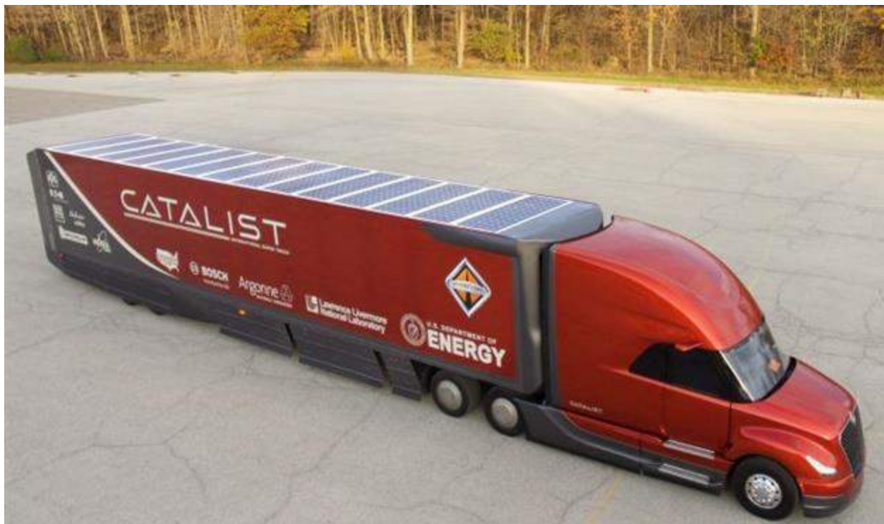
The fuel-efficiency SuperTruck concept truck from Navistar used solar panels extensively. Volvo’s SuperTruck used them as well. Photo: eNow
