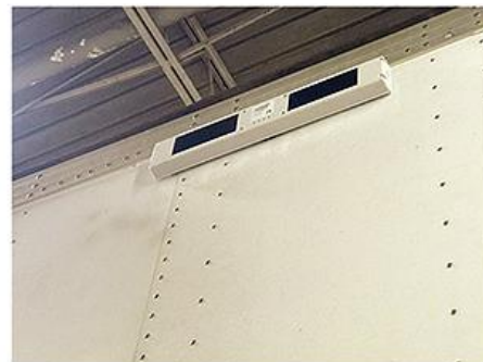
A solar-powered tracking system from SkyBitz installed on a trailer. (SkyBitz)
